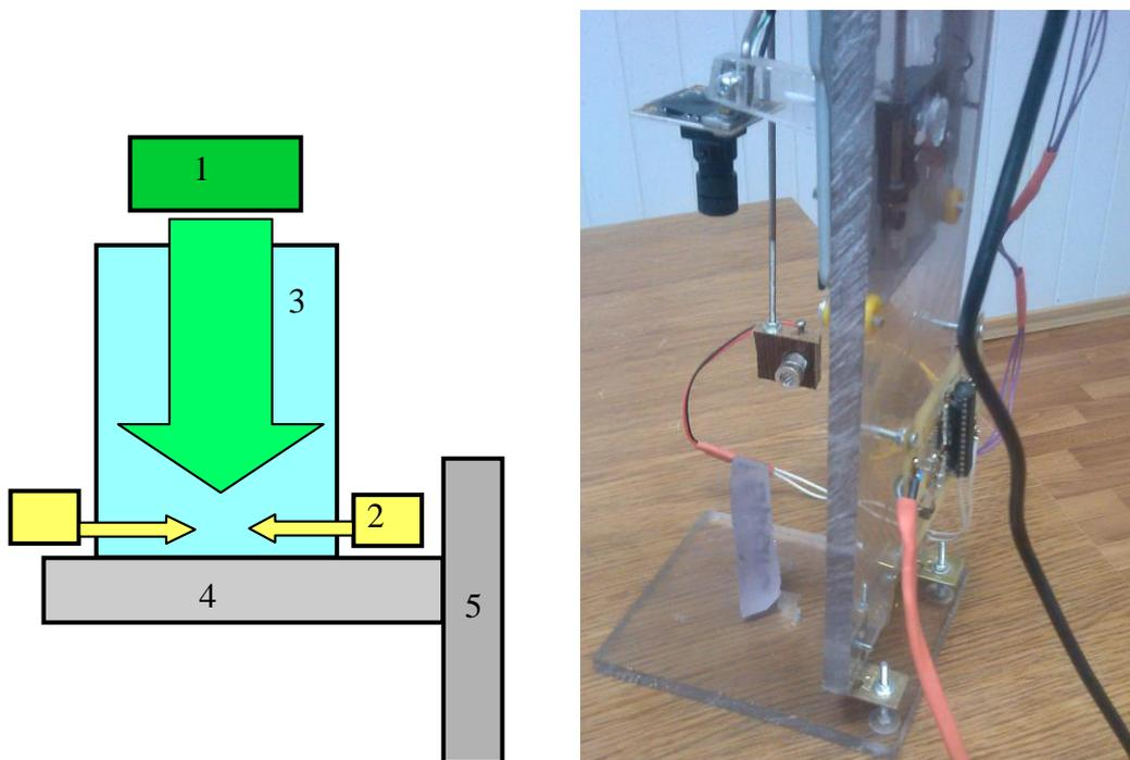
**Figure 1: The scheme and the facility appearance; 1 – camera; 2 – the lights; 3 – crystal; 5 – table; 6 – incremental driver**
