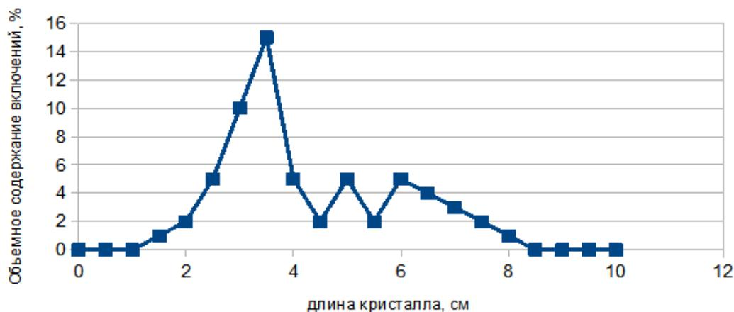
**Figure 3: Inclusions dispersion through the crystal's length**
